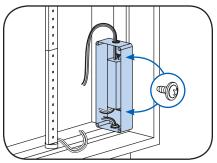
1 Mount the power supply. Mounting the power supply base directly to a thermally conductive installation surface can improve thermal performance.
