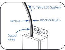
3 Connect the supply wire that is attached to the Tetra LED System to the red (+) and black or blue (-) output wires of the power supply as outlined in the "Electrical Connections" section of your LED system's Installation Instructions.
