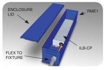
The RME1 enclosures accepts "B" configuration ILB-CP units for remote mounting. The ILB-CP is secured within the enclosure and wiring is routed through the 2 ft. of flexible conduit for connecting to the fixture. Can be used in conjunction with the TBMK for grid ceiling mounting.
