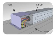
When top-mounting "B" configuration ILB-CP units, the TMK-32 is used to cover the exposed wiring that goes from the battery pack into the fixture.
