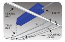
Use the TBMK mounting kit to remote mount flexed units within a grid ceiling. The ILB-CP is secured to the bars of the TBMK via mounting clips. The bars then mount to the T-bars of the ceiling grid. The flexible conduit of the ILB-CP connects to the fixture.
