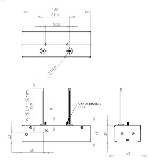
Dimensions for all the diagrams are in mm and are for reference only. For exact dimensions and tolerances, refer to the 3-D models (.STEP files) for the LMD800 driver available by selecting the Documentation tab on the LMH2 product page.
