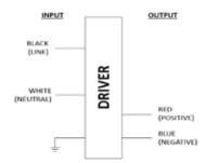
Input and output use lead- wires.
