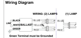
The wiring diagram that appears above is for the lamp type denoted by the asterisk  $(\ensuremath{^*})$
