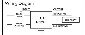
Input, Output and 0-10V Dimming use lead-wires. Lead-wires are 18AWG 105C/600V solid copper
